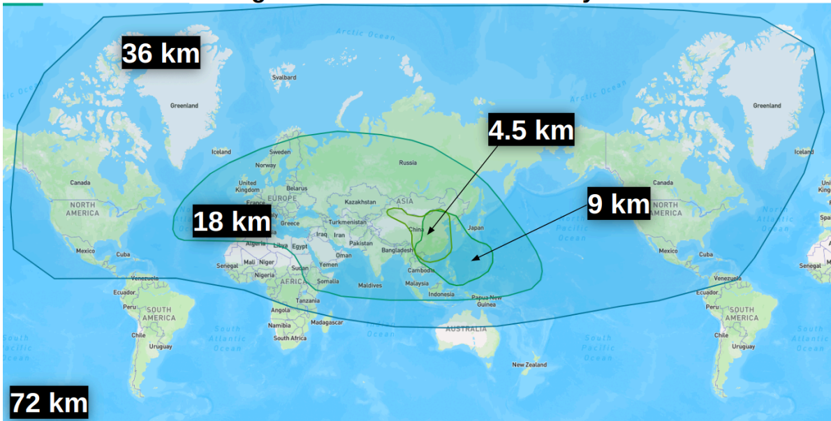
Figure 1: The mesh resolution of CPAS daily run. The resolution for TCs in the Western North Pacific and part of China is 9 km and 4.5 km respectively, and the outermost domain is 72km.
